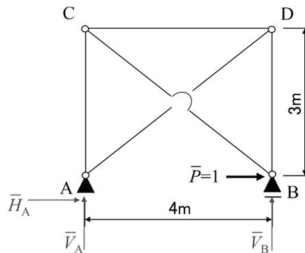
$$\begin{aligned} \sum H &= \bar{H}_A + 1 = 0 \\ \sum V &= \bar{V}_A + \bar{V}_B = 0 \\ \sum M_{(A)} &= \bar{V}_B \cdot 4 = 0 \end{aligned}$$
