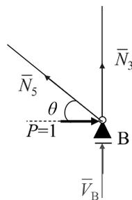
$$\begin{aligned} \sum H &= \bar{N}_5 \cos \theta - 1 = 0 \\ \sum V &= \bar{V}_B + \bar{N}_3 + \bar{N}_5 \sin \theta = 0 \end{aligned}$$
