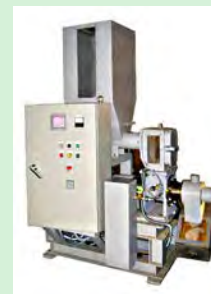
Expansion softening device 膨張軟化処理装置
