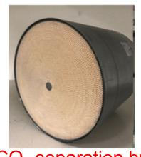
CO<sub>2</sub> separation by honeycomb wheel
